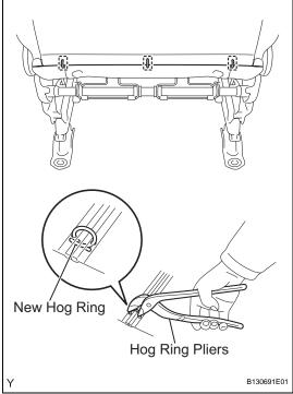
(g) Using hog ring pliers, install 3 new hog rings.
